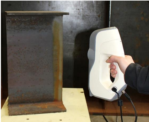
FIGURE 2. Use of the Artec Eva for scanning corroded beam in UCONN Structures Laboratory
